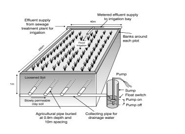
during heavy rainfall and low evapotranspiration periods, obviating the need for expensive storage. Effluent flow rates through the soil profile, and the depths of the watertable in the FILTER plots are controlled through regulated pumping from sumps. During this regulated flow of effluent, nutrients are adsorbed on the surface of soil particles or taken up by the crop and weeds.
